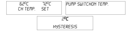
This option can be used to set the hysteresis of the set temperature. It is the difference between the temperature of start of the suspension mode and the temperature of restarting the operation mode (e.g. when value of the set temperature is 60°C and hysteresis is 2°C, the start of the suspension mode will take place at 60°C, whereas the restart of the operation mode will take place at 58°C. Hysteresis can be set in the range between 2°C and 6°C.
