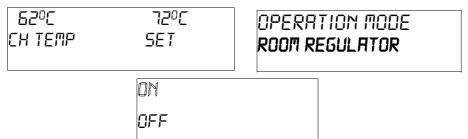
**ST-81** thermo regulator allows a room regulator to be connected in the system. In this mode the thermo regulator is being controlled by the room regulator and does not take into account the temperature set on thermo regulator main unit. Blow is operating until the temperature set on the room regulator is reached. However the operation of the boiler is limited by the temperature set on the thermo regulator mounted on the boiler.
