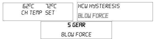
This function allows to choose the operations speed of the fan. Range of regulations is between 1 and 10 (one can assume those are the gears of the fan). The higher the gear the faster the operation of the fan, whereas gear 1 is the minimal speed and gear 10 is the maximal speed. Change of gears is being done by the means of PLUS and MINUS buttons. The fan always starts up with the maximal speed which allows it to start operation even with some amount of dust present in the engine.
