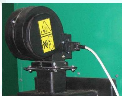
Fig.13. a) view of the blower (cast-iron type), b) blower plug, c) identification of connection terminals.
